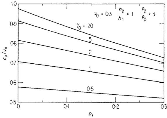
FIG. 6. Wave speed vs. porosity.
