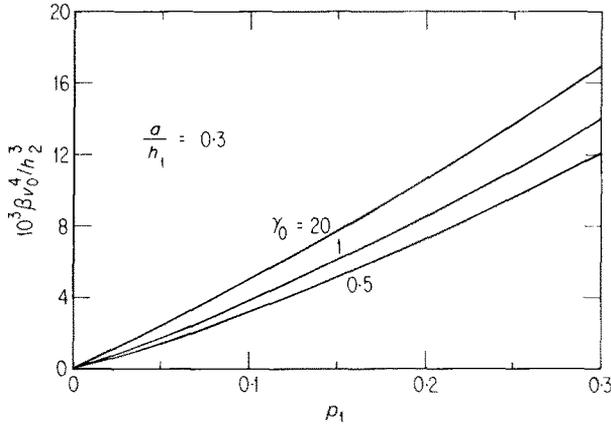
FIG. 8. Attenuation parameter vs. porosity.
