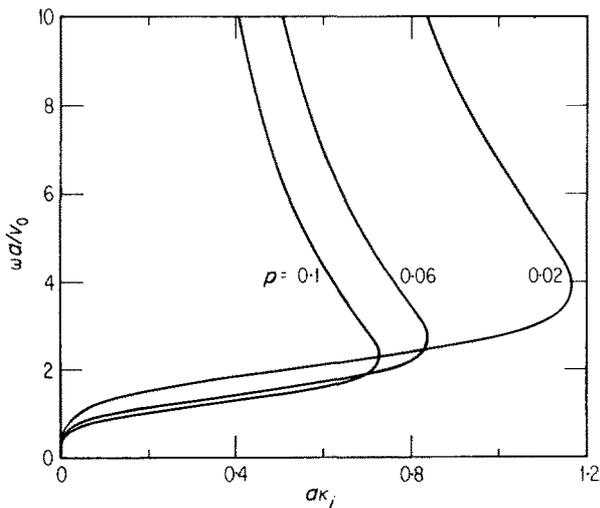
FIG. 4. Frequency vs. imaginary part of wave number for porous medium.
