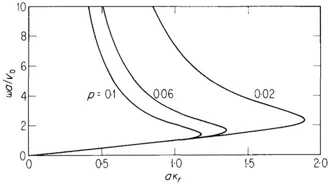
FIG. 3. Frequency vs. real part of wave number for porous medium.
