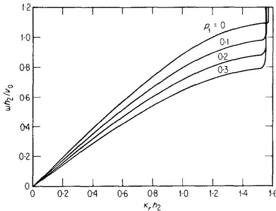
FIG. 9. Frequency vs. real part of wave number for porous composite.
