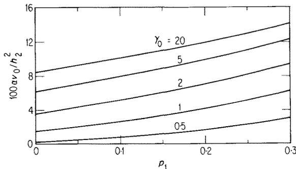
FIG. 7. Dispersion parameter vs. porosity.
