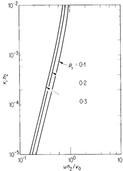
FIG. 10. Imaginary part of wave number vs. frequency for porous composite.
