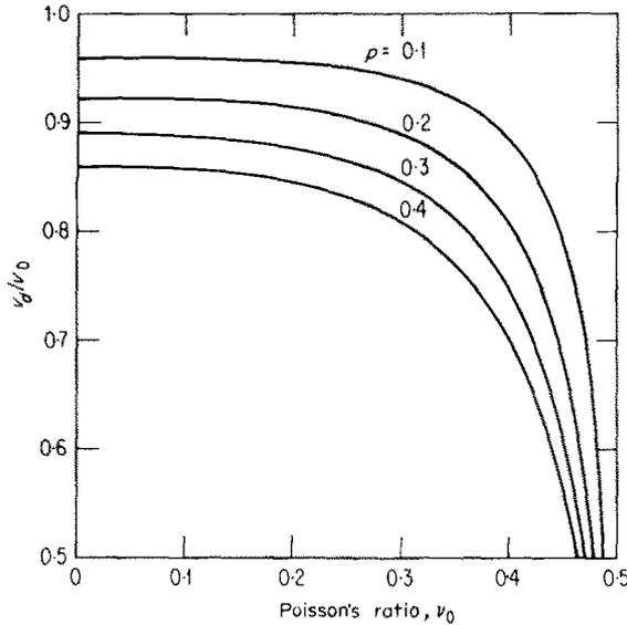
FIG. 1. Effective wave speed vs. Poisson's ratio.
