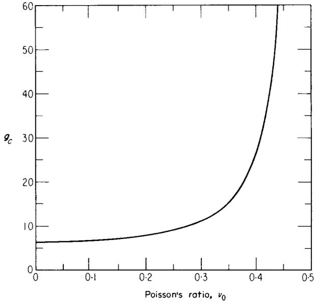
FIG. 2.  $g_c$  vs. Poisson's ratio.
